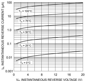
V<sub>R</sub>, INSTANTANEOUS REVERSE VOLTAGE (V) Fig. 4 Typical Reverse Characteristics
